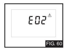
The control has detected no increase in the supply water temperature within the BOIL Alarm time setting. Check to see if the boilers are operating properly using the Test button. To reset the alarm, press and hold the up and down arrow buttons for 5 seconds while in the VIEW menu.
